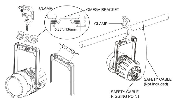
ENSURE ALL CONNECTIONS AND END CAPS ARE PROPERLY SEALED WITH A DIELECTRIC GREASE (AVAILABLE AT MOST ELECTRICAL SUPPLIERS) TO PREVENT WATER CORROSION AND/OR ELECTRICAL SHORT CIRCUIT.
